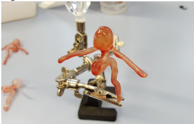
Hollow Dynamic Patient-specific aneurysm pathology used in the 4D simulator for training aneurysm clipping procedure
