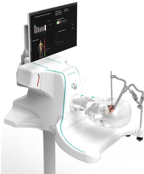
4D Simulator with patient-specific head model for training complex aneurysm treatment procedure
